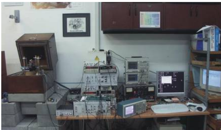
Figure 0.4. PRONANO experimental cantilever control and data acquisition system
