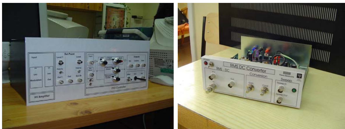
Fig. 0.2: Analogue PID controller (left) and high-speed RMS/DC converter (right)
